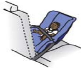
Alternate seat belt position for the rear facing infant seat depending on make and year of car and model of car seat
